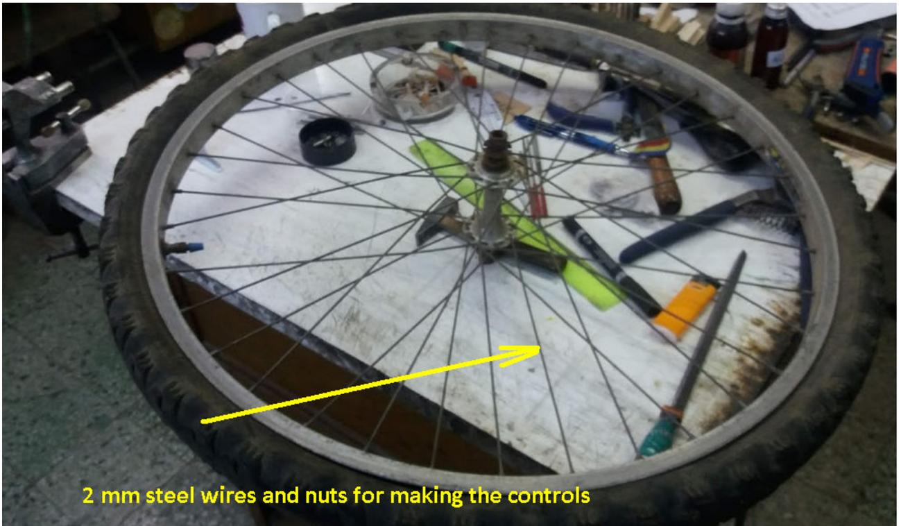
2 mm steel wires and nuts for making the controls
